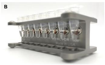
**Figure 3: Magnetic racks for CUT&RUN assays. (A)** For batch processing of ConA beads, use a 1.5 mL magnetic rack (*e.g.* EpiCypher 10-0012, pictured). **(B)** For processing samples in 8-strip PCR tubes we recommend using a multi-channel pipette and compatible magnetic rack (*e.g.* EpiCypher 10-0008, pictured).
