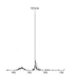
**Mass Spec Data:** Synthetic H3K27me3 protein analyzed by ESI-TOF mass spectrometry. Expected mass = 15,314.97 Da. Determined mass = 15,314.45 Da.
