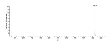
Mass Spec Data: H4K12me1 protein analyzed by high resolution mass spectrometry. Expected mass = 11,291.15 Da. Determined mass = 11,291.35 Da.
