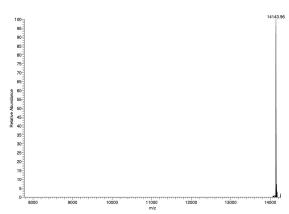
Mass Spec Data: Synthetic H2AK5,9,13,15ac histone analyzed by ESI-TOF mass spectrometry. Expected mass = 14,144.29 Da. Determined mass = 14,143.96 Da.
