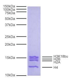
**Protein Gel Data:** Coomassie stained PAGE gel of proteins in Nucleosome, Recombinant Human, H3K18bu (1  $\mu$ g) to demonstrate the purity of the histones in the preparation. Sizes of molecular weight markers and positions of the core histones (H2A, H2B, H3K18bu and H4) are indicated.
