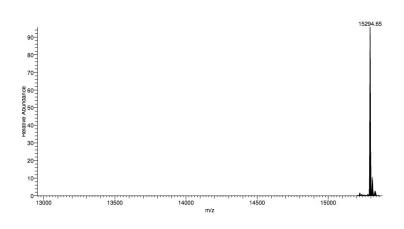
**Mass Spec Data:** H3K18bu protein analyzed by high resolution mass spectrometry. Expected mass = 15,294.8 Da. Determined mass = 15,294.7 Da.
