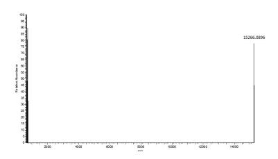
**Mass Spec Data:** H3K4ac protein analyzed by high resolution mass spectrometry. Expected mass = 15,266.8 Da. Determined mass = 15,266.1 Da.
