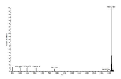
**Mass Spec Data:** H3K4me3, K9,14,18ac protein analyzed by high resolution mass spectrometry. Expected mass = 15,389.8 Da. Determined mass = 15,391.5 Da.
