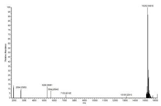
**Mass Spec Data:** Synthetic H3K4me2 histone analyzed by high resolution mass spectrometry. Expected mass = 15,252.8 Da. Determined mass = 15,252.5 Da.
