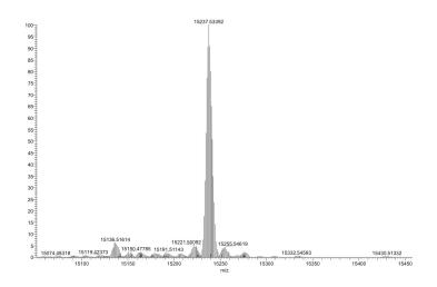
**Mass Spec Data:** Synthetic H3 K4Me1 protein analyzed by ESI-TOF mass spectrometry. Expected mass = 15,238 Da. Determined mass = 15,237.5 Da.
