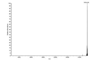
**Mass Spec Data:** Synthetic H3K27me3 histone analyzed by high resolution mass spectrometry. Expected mass = 15,314.97 Da. Determined mass = 15,314.45 Da.
