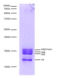
**Protein Gel Data:** Coomassie stained PAGE gel of proteins in H3K27me3 dNuc (1  $\mu$ g) to demonstrate the purity of histones in the preparation. Sizes of molecular weight markers and positions of the core histones (H2A, H2B, H3K27me3 and H4) are indicated.
