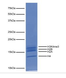
FIGURE 3 Protein gel data. Coomassie stained SDS-PAGE gel of proteins in H3K4me3 dNuc (1  $\mu$ g) demonstrates the purity of histones in the preparation. Sizes of molecular weight markers and positions of the core histones (H2A, H2B, H3K4me3 and H4) are indicated.
