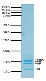
**Protein Gel Data:** Coomassie stained PAGE gel of proteins in Nucleosome, Recombinant Human, H3K9ac (1  $\mu$ g) to demonstrate the purity of the histones in the preparation. Sizes of molecular weight markers and positions of the core histones (H2A, H2B, H3K9ac and H4) are indicated.
