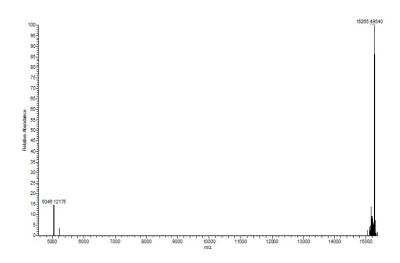
**Mass Spec Data:** H3K9ac protein analyzed by high resolution mass spectrometry. Expected mass = 15266.8 Da. Determined mass = 15,265.5 Da.
