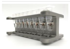
FIGURE 2 CUTANA™ CUT&RUN 8-strip 0.2mL tubes. 8-strip 0.2 mL tubes are compatible with the Magnetic Separation Rack (EpiCypher 10-0008) for use during all bead separation steps in the CUT&RUN procedure, including sample immobilization with ConA beads and library preparation. Magnetic Separation Rack is not included in the purchase of this product.
