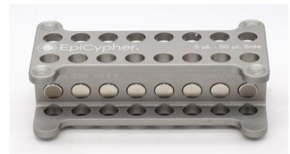
Figure 2. For ConA bead activation steps, it is recommended to batch process the full volume of beads needed for all experimental samples in a single 1.5 mL tube (11 \mu\text{L} beads per sample). For these steps, beads can be washed using a 1.5 mL magnetic rack (e.g. EpiCypher 10-0012, pictured), ensuring homogeneity across samples.
