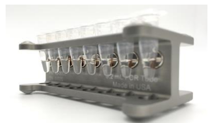
Figure 3. For processing individual samples, it is recommended to use multi-channel pipetting using 8-strip PCR tubes and compatible magnetic rack (e.g. EpiCypher 10-0008, pictured), increasing experimental throughput and reproducibility.
